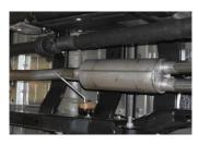
**3.** Install muffler #B onto head pipe #A  $1\frac{1}{2}$ "-2" with the louvers facing towards the converter and muffler outlets level. Use a jack stand to support the muffler. Use clamp #G to secure the muffler to the headpipe. Do not tighten. Muffler inlet is looking into the louvers.
